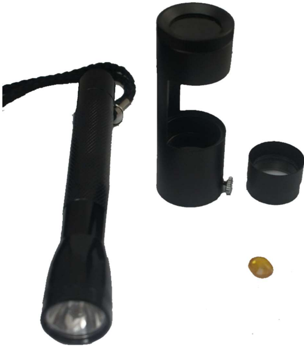
Photo 3.5: L-R Torch, Upper and lower polaroids, Stone-table
