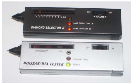
Photo 5.4: Upper Diamond selector. Lower Moissanite and Diamond differentiator.
