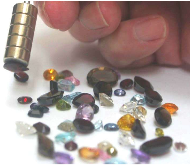
Photo 2.2: The magnet spear has lifted a red stone, (a garnet), from the selection shown earlier.
