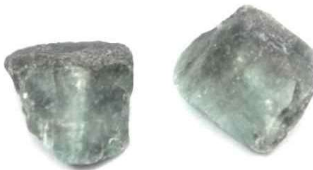
Photo 1.19: Two natural part crystals of Emerald showing the 120^\circ angle between faces.
