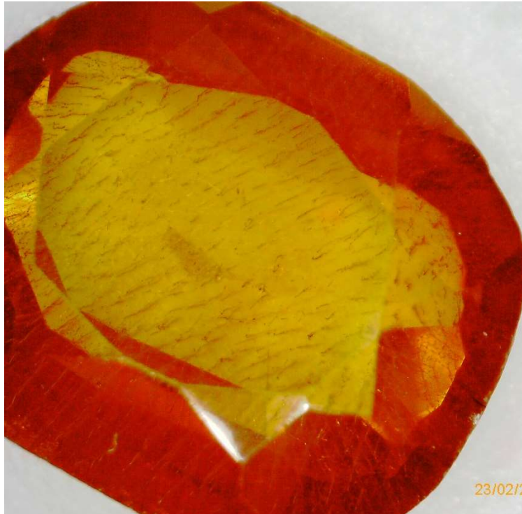
Photo 7.17: Straight colouring lines in a Sri Lankan 8 carat yellow natural Sapphire.
