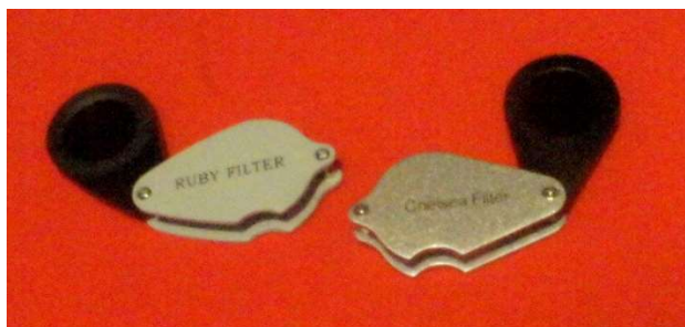
Photo 6.4 Left: Glass Ruby Filter and Right: Chelsea Filter
