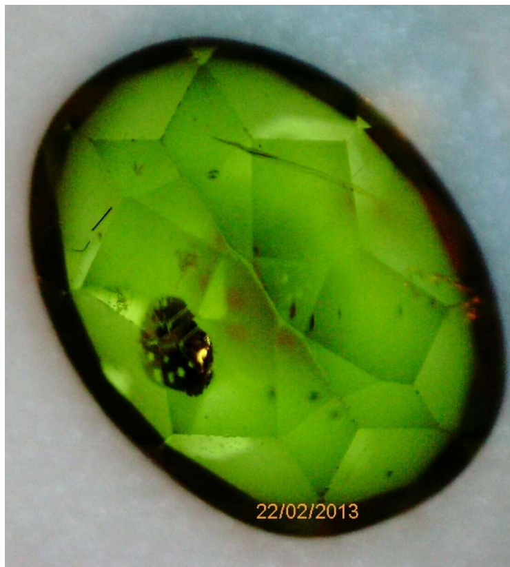
Photo 7.8: Peridot 1.65ct Colour Change with a large solid inclusion
