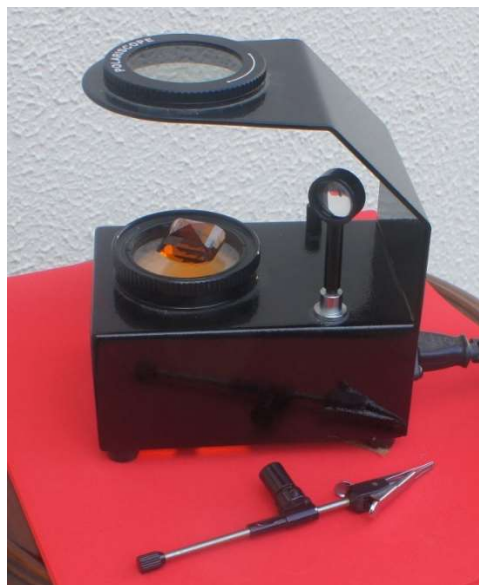
Photo 3.2: Desk Polariscope with Conoscope converter in holder and stone holder (detached)
