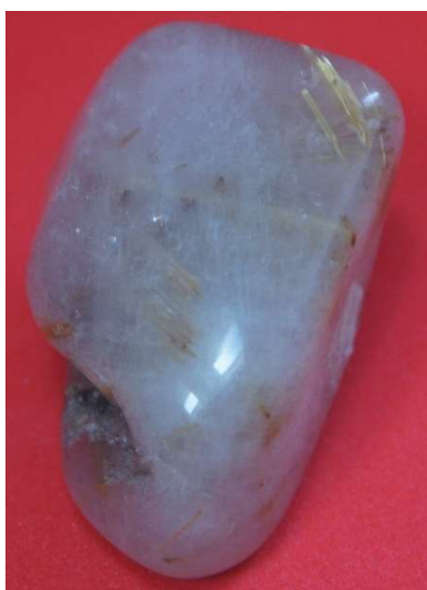
Photo 1.13: Quartz with golden rutile (Titanium Dioxide) needle Inclusions.
