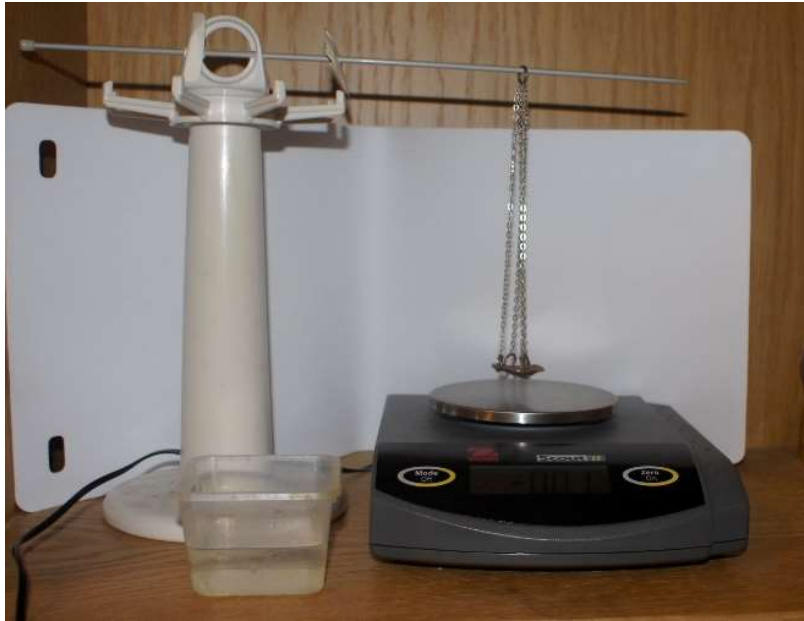
Photo 2.5: Apparatus for Specific Gravity test.
