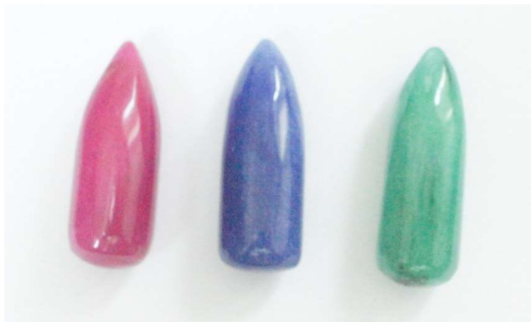
Photo 5.6 Three Boules of Verneuil process Spinel.
