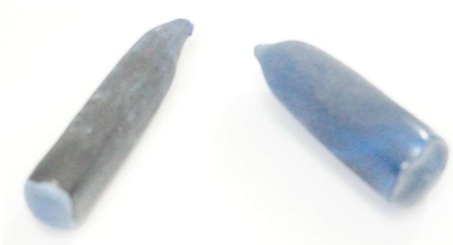
Photo 5.8 Two Boules of Synthetic Spinel from which Sapphire simulants are cut..
